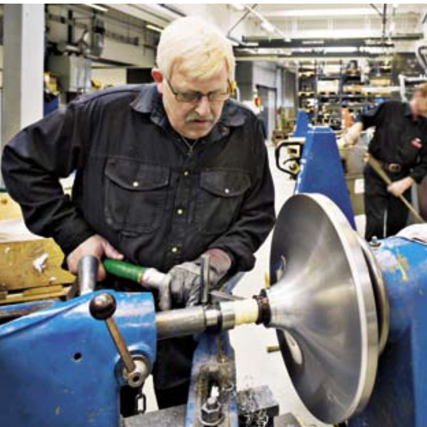
Louis Poulsen's factory combines artisan traditions with cutting-edge technology. The metal shades are hand pressed, all fixtures are assembled manually and painted components are sprayed by hand or powder-coated.
