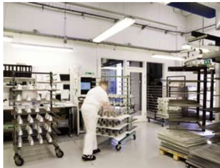
Louis Poulsen's factory combines artisan traditions with cutting-edge technology. The metal shades are hand pressed, all fixtures are assembled manually and painted components are sprayed by hand or powder-coated.
