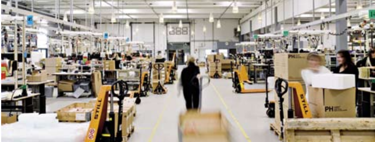
Staff assemble the products in cells, usually with two or three people looking after assembly, testing and packaging.
